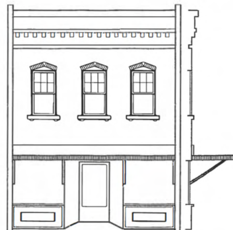
Figure 115: Examples of inappropriate metal and vinyl awnings.
